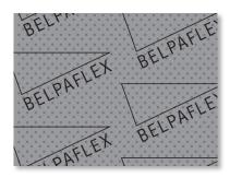
Belpaflex comprises two asbestos free paper sheets assembled around a central rectangular perforated steel sheet. It is suitable for use in high temperture resistant cylinder head gaskets and exhaust manifold gaskets on petrol and diesel engines and is resistant to oil, fuel and cooling mixture.
