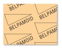
Cellulose based material impregnated with plasticised gelatine. Very economical material with excellent oil and fuel resistance, its main market is automotive. This material must be protected from sudden changes in humidity and temperature to prevent dimensional changes.
