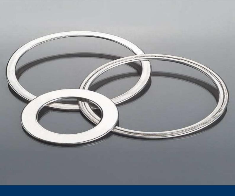
Metal Jacketed gaskets are used for high pressures and temperatures. The metal coating gives resistance and protects against corrosion, while filling gives soft material resilience. They are specially designed for boilers and heat exchangers and allow its use in very narrow surfaces. The determination of metal material and filling material will be based on fluid and temperature must withstand the seal.
