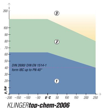
\*Gaskets according to DIN 2690 are only standardised up to PN 40
